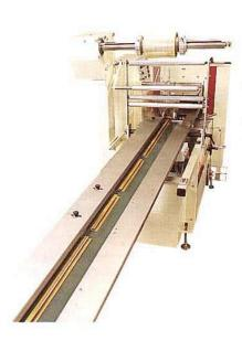
Products of varying length can be automatically overwrapped
