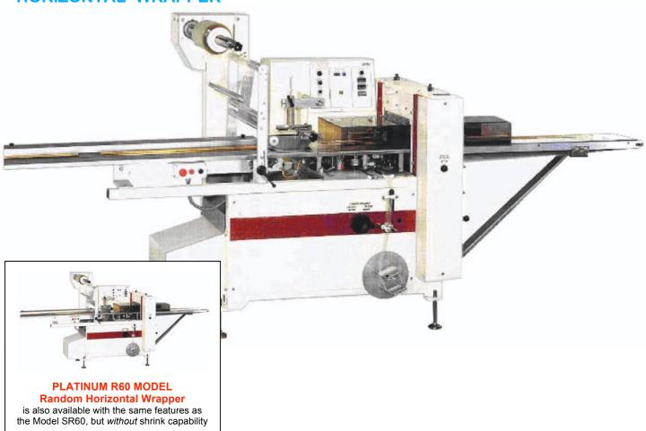
Platinum's SR60 Model Random Length Horizontal Shrink Wrapper is specifically designed to overwrap products such as window shades, molding, loaves of bread and specialty tubing which are consistent in terms of height and width, but may vary in length.
