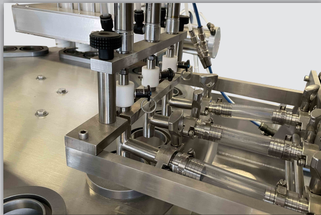
Quick Release Filler / Easier For Changeover Or Cleaning
