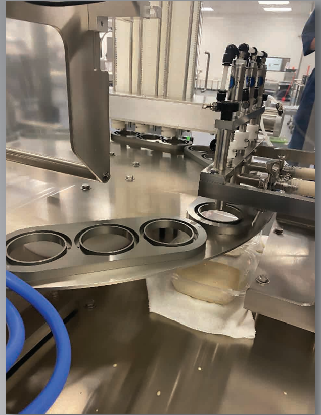
Access Frame & Top Plate 3/8" & 16 G Stainless Steel
