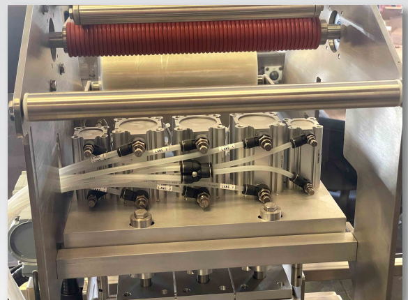
Quick Release Heat-Seal / Tooling Without The Use Of Tools
