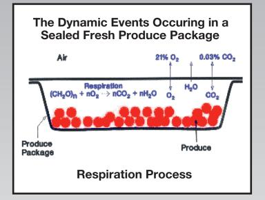
gy is based on patented technology that uses lasers to register microperforations in a well-defined area on the package so that OTRs are maintained at desired levels during storage and shipment. These films are customized for your particular produce item and weight, creating an optimum atmosphere that will go a long way toward maximizing freshness and shelf life.
