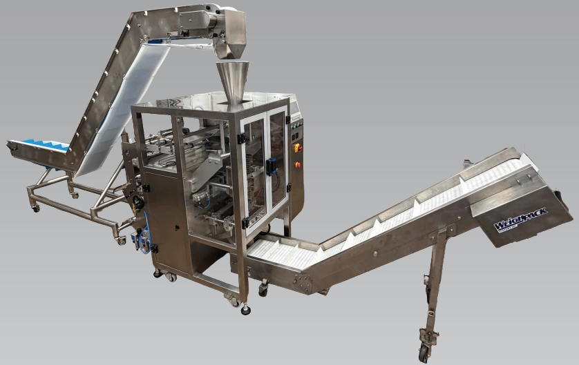
In Line 'I' Shaped Infeed System for the Platinum VB Bagger
